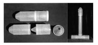
FIG. 1. Shrimp funnel trap components (left) and modified inverted "T" design (right). The upright vertical air circulation pipe allows snakes access to air.
